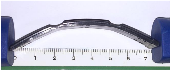
Figure 1: Sliding strip SV35 – maximum arch bending (7,5 cm)
