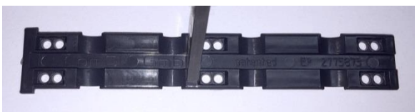
Figure 4: Sliding strip SV55 – maximum reverse bending (straightened)
