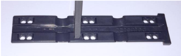
Figure 2: Sliding strip SV35 – maximum reverse bending (straightened)
